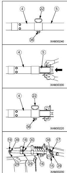
8. Slide storage bar (16) to the direction of the head of main boom.
