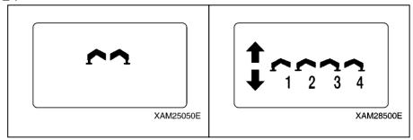
2. Push Speed/Mode button in the mode condition of above 1. The operation mode is switched to "Outrigger Extension mode".
