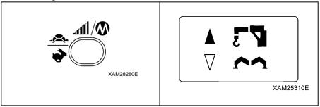
4. Use the Hook raising and lowering Lever and shift the cursor (▲ or ▼), and push the Setting button when the cursor points out the "OUTRIGGER".
