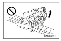
• The rubber tracks slip very easily on a wet steep plate or snowed and frozen surface. Be especially careful not to slip when operating on the slope.
