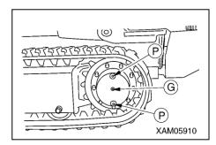
3. If there is no sufficient oil, remove the top drain plug (P) and pour in gear oil from the plug hole.
