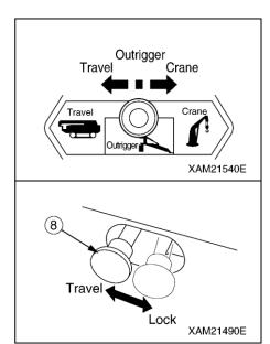
2. Push down the traveling lock levers (8) to the "TRAVEL" position.
