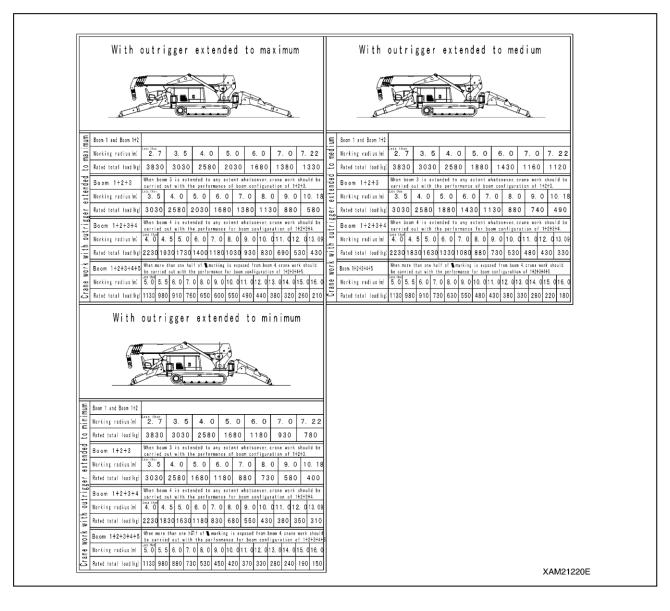
The rated total load chart provides the maximum loads that the crane is capable of hoisting objects in parallel with the length of the boom. The loads are specified by working radius.
