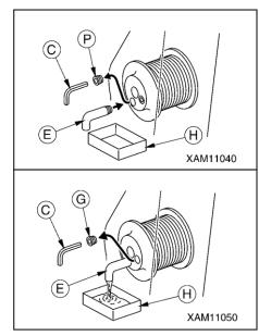
11. Pump the gear oil through the oil inspection plug (G) with the use of the oil pump (D).
