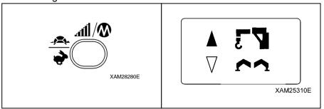
3. Use the Hook raising and lowering Lever and shift the cursor (▲ or ▼), and push the Hook stow/Setting button when the cursor points out the "OUTRIGGER".
