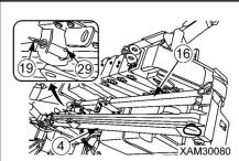
4. Lift up No.1 Fly-jib (4) tip to take it out from stow stay, then slew it around the position pin (17) (length: 150mm) on the right side of the head of main boom.
