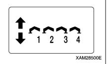
6. Turn one of the outrigger operation levers to "Extend (lower)" and pull the Accelerator lever slowly.
