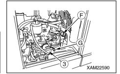
10. Clean the filter stand. Apply clean engine oil (or a light coating of grease) to a new filter cartridge gasket and thread part, and install the filter cartridge.
