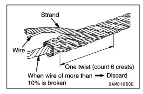
Wear equivalent to 7% or more of a nominal diameter occurs in the wire rope diameter.
