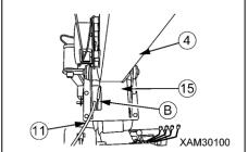
11. Hang attachment lever block (28) between No.1 Fly-jib bracket (32) and bracket (2).
