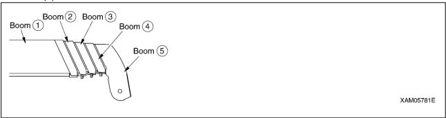
2. "Boom (1) + (2)": With booms (3), (4), and (5) retracted, boom (2) is fully extended. "Boom (1) + (2)" is to apply to crane operation with boom (2) extended even if only slightly.
