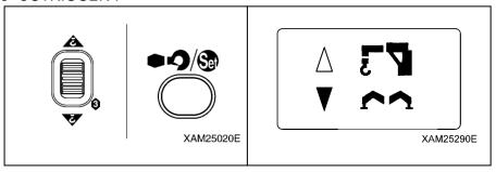
Here, confirm that the "Outrigger mark" is exhibited, then it enters into the "Ground setting mode", soon
