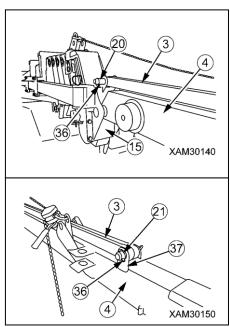
16. Move two supporting rods (3) to bracket (2) on the head of main boom and put position of the hole together.
