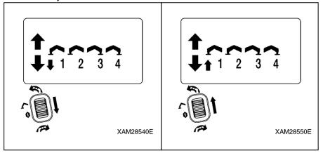
6. To shift to "Extension mode", push the Speed/Mode button, while the LCD screen shows the "Ground setting mode".
