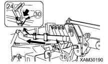
23. Insert position pin (18) (length: 55mm) into the hole of stopper (30) on the center of storage bar (16), and lock position pin (18) firmly by linch-pin (29).
