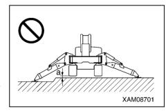
The machine becomes unsteady at some point if it undergoes a 360-degree slewing with an object hoisted. Irrespective of the rated total load, ensure operation in a short working radius and at low speed.
