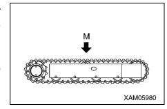
3. Measure the clearance between the wheel tread of the track roller at center and the shoulder of the rubber track.
