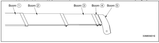
4. "Boom (1) + (2) + (3) + (4)": With booms (2) and (3) fully extended, booms (4) and (5) are extended midway (half of the " ■ mark" passes boom (3)).
