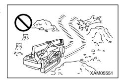
At the location where there are great amount of large and small boulder stones such as river beds, the stones will go under the machine, tending to damage the rubber tracks or the rubber tracks tend to come off.
