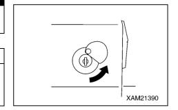
Use this switch to start and stop the electric motor.
