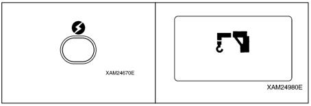
2. While the "Crane mark" is shown in the LCD screen (for approx. 2 seconds), push the Speed/Mode button for 2 seconds.
