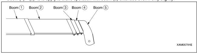
3. "Boom (1) + (2) + (3)": With booms (4) and (5) retracted, booms (2) and (3) are fully extended. "Boom (1) + (2) + (3)" is to apply to crane operation with boom (3) extended even if only slightly.
