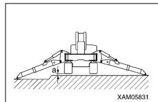
The figure shown at right represents the condition "When the crane is used with the outriggers extended at the maximum" in the rated total load chart.
