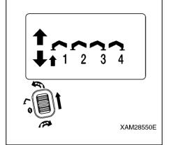
4. Push Speed/Mode button in the mode condition of above 3. The operation mode is switched to "Outrigger Extension mode".
