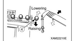
4. With the boom stowing switch knocked to the "ON" position, operate the boom derricking lever (4) again to the "LOWER" (push forward) side to stow the boom.
