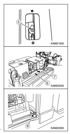
16. Start the engine with the drain valve (8) open, and ensure the engine runs at low idle. Conduct a cleaning with running water until clean water flows out of the radiator.
