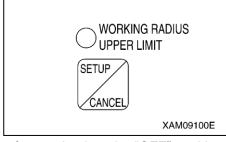
To enable this setting, turn the key switch to the "ON" position again after turning it to the "OFF" position, or reduce the working radius by "1.3 m" or more from the set working radius to get out of the pre-warning zone while the engine is being started.
