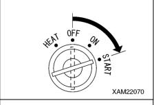
3. Release your hand from the key once the engine has started. The key will automatically return to the "ON" position.
