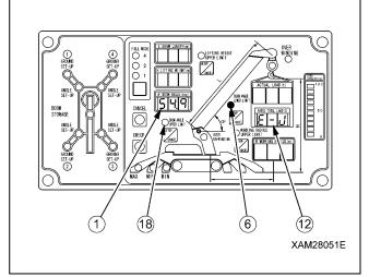
(When the boom length is 12.5m or less, the boom can be lowered for the purpose of stowing boom.) In such event, raise the boom to the safety range from restricted zone.
