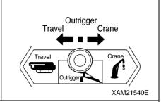
Push Fall mode selector switch (1) for 2 seconds or more. Operation mode will change as shown below. Keep in mind that the switch should be released and re-pushed to proceed to next mode.
