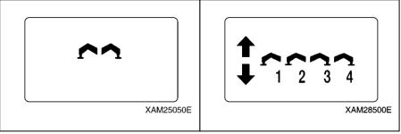
5. To shift to "Extension mode", push the Speed/Mode button, while the LCD screen shows the "Ground setting mode". Then the mode is switched to "n"; the mark turns to "Extension (← →)".
