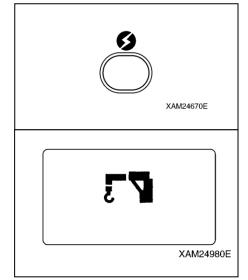
3. While the "Crane mark" is shown in the LCD screen (for approx. 2 seconds), push the Speed/Mode button for 2 seconds.
