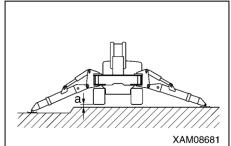
The figure shown at right represents the condition "When the crane is used with the outriggers extended midway" in the rated total load chart.
