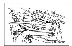
2. Move No.1 Fly-jib (4) and storage bar (16) to the direction of head of the main boom.
