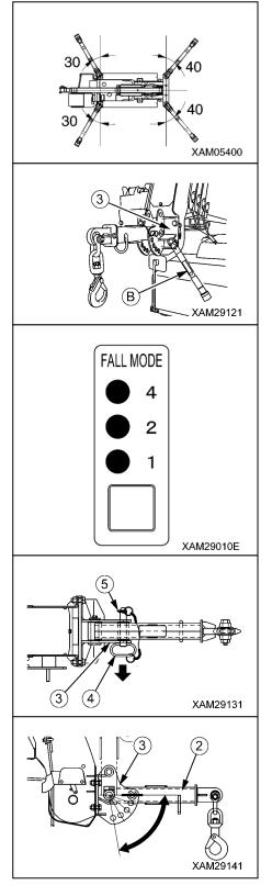
6. Insert the position pin (4) through the hole of bracket (3), and secure it with the snap pin (5) to the tip of position pin (4).
