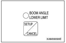
To enable this setting, turn the key switch to the "ON" position again after turning it to the "OFF" position, or raise the boom by "7 degrees" or more from the set boom angle to get out of the pre-warning zone while the engine is being started.
