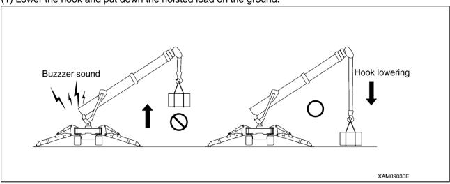
(2) Raise the boom. Lower the hook so that the hoisted load will be as low as possible.
