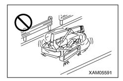
• Do not operate the machine in a way that the edge of the rubber tracks is pressed against the concrete and walls.
