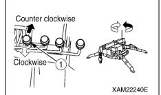
3. Operate the boom derricking lever (4) to the "LOWER" (push forward) side and lower the boom until it automatically stops.
