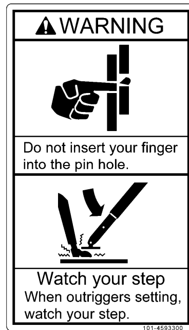
(28) Outrigger pin hole caution and footing check (101-4593300) (4 places)
